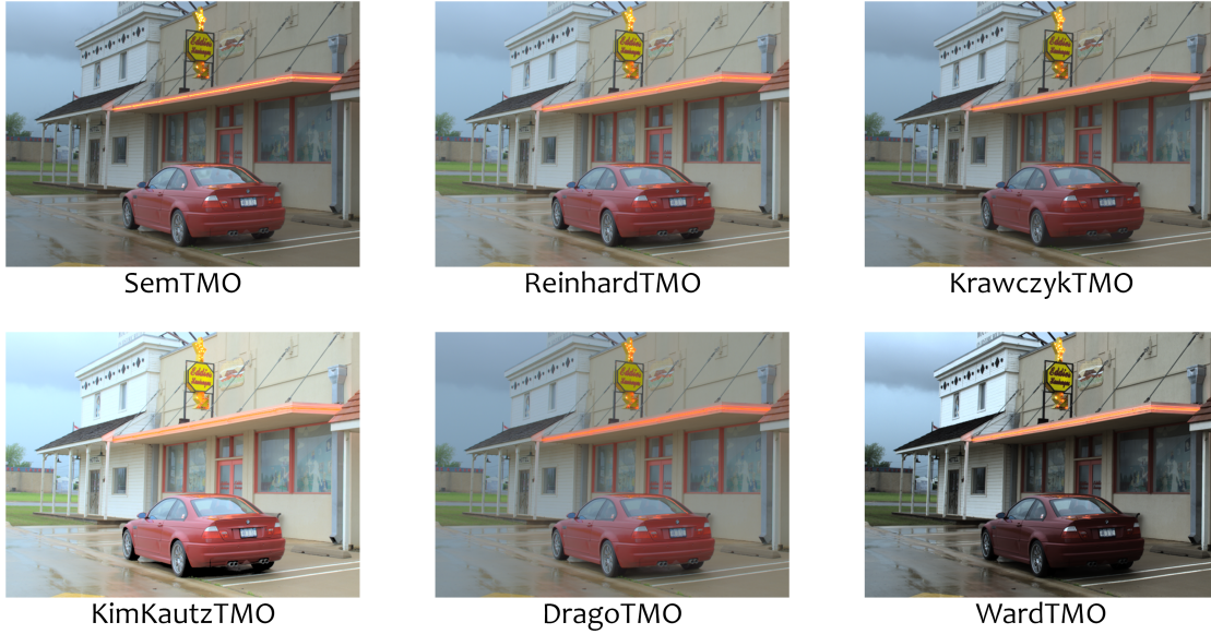
Figure 1.4 – Output of 6 TMOs for the same scene.
