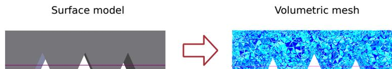
Figure 3.3: Illustration of a mesh. The volumetric mesh is created from a surface model of the manipulator.
