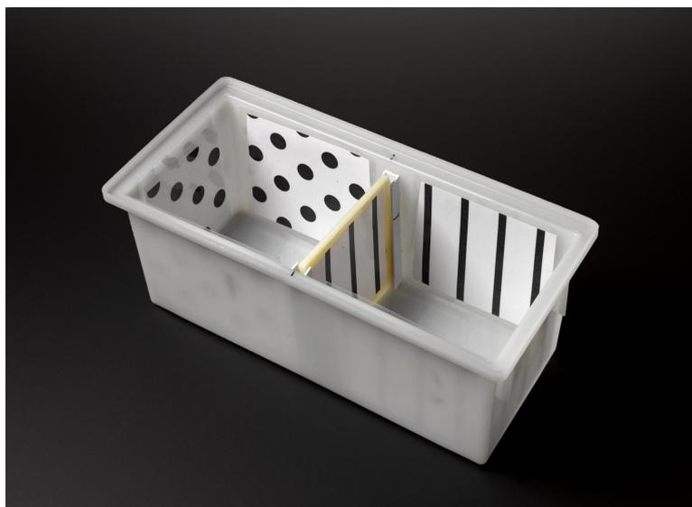
**Figure 6.5 – Conditioned place preference apparatus.** CPP setup for zebrafish reproduced from Brennan Caroline, Queen Mary University of London. The middle wall is removed for the first and third step of the CPP.
