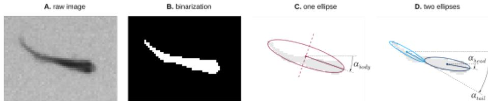
**Figure 3.3 – Detection** Details of the detection phase for one object of the movie *ZFJ\_001*. **(A)** raw image. **(B)** binarized image obtained by subtraction the background image and applied a threshold. **(C)** equivalent ellipse of the object. **(D)** two equivalent ellipses, useful for a deformable object.
