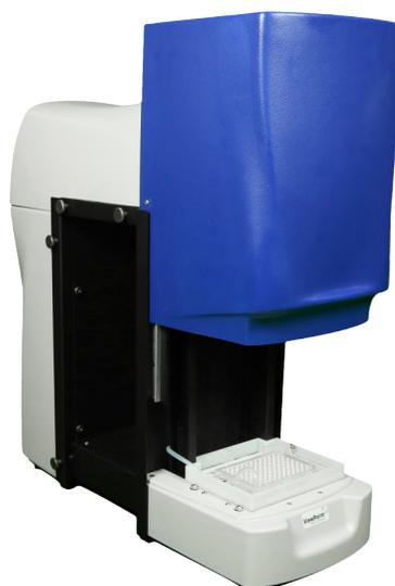
**Figure 6.6 – A Zebrabox from Viewpoint.** Zebrabox, the most used solution for well-plates experiments.
