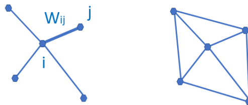
Figure 3.18 – Example of representation of irregular grid data. On the left: an undirected graph. On the right: a mesh.
