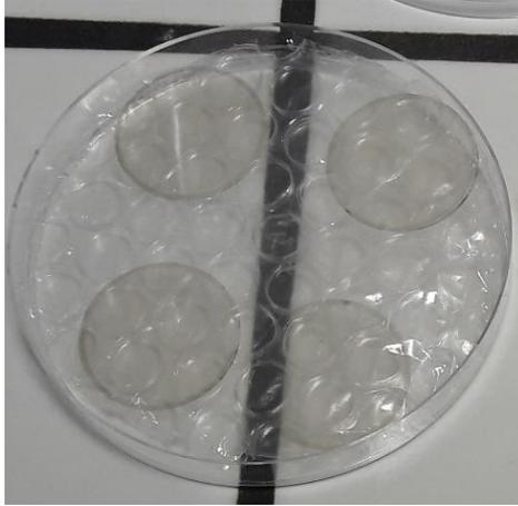
Figure V.1: Ag:TiO<sub>2</sub> films deposited on four circular flexible glass. The photographs were taken after the three UV-VIS cycle.
