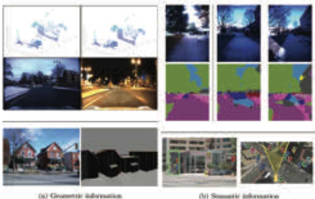
Figure 2.4: Illustration of the data heterogeneity in VBL: 2.4(a) From top to bottom: PointNetVLAD [304] used to match point cloud for VBL and localization system built upon a DEM [179]. 2.4(b) From top to bottom: data segmentation to help queries (right) to database (left) visual association [272] and localization systems with semantic information gathered from OpenStreetMap annotation [7].
