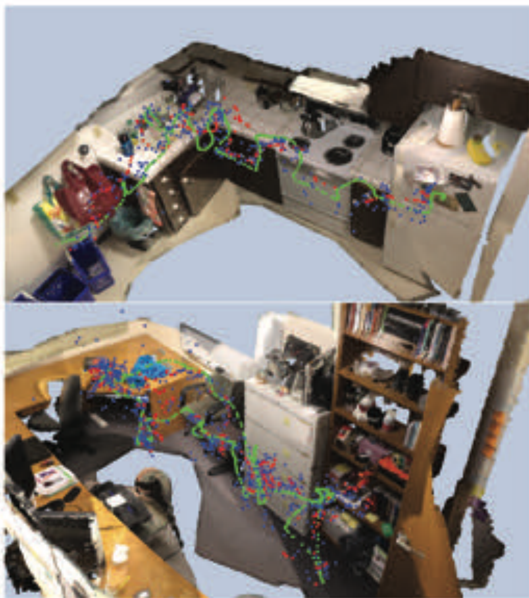
Figure 4.4: Visualisation of the refined camera position: ground truth positions of test sequences are marked in green, initial position from image indexing in red and refined position after PnP in blue. Environment from the I2 scenes dataset [108]: top apartment 1-kitchen and bottom music.
