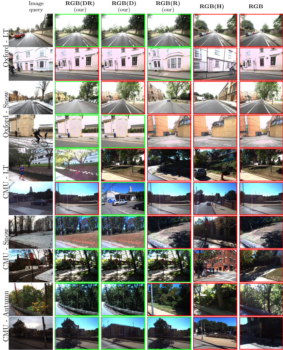
Figure 3.15: Comparison of top-1 retrieved images: we show top-1 retrieved candidate after the nearest neighbor search for the different descriptor. Red box indicates a wrong match and green box a proper one ( i.e. retrieved image lies in 25m radius from the query ground truth position). All the descriptor use Resnet18 as backbone, excepted RGB(H).
