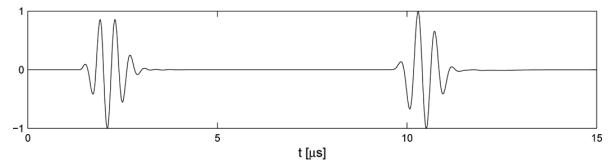
Fig. 8. Example of signal generated from the matrix  $\mathbf{G}$  in Fig. 7. The data  $\mathbf{y}$  are computed from the columns 200 and 1000 of matrix  $\mathbf{G}$  such that:  $\mathbf{y} = \mathbf{g}_{200} + \mathbf{g}_{1000}$  where  $\mathbf{g}_i$  is the  $i$ th column of  $\mathbf{G}$ . Both echoes are normalized in amplitude for visualization clarity.
