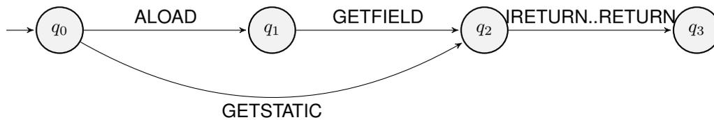
Figure 2.2: Finite automaton to detect simple getter methods
