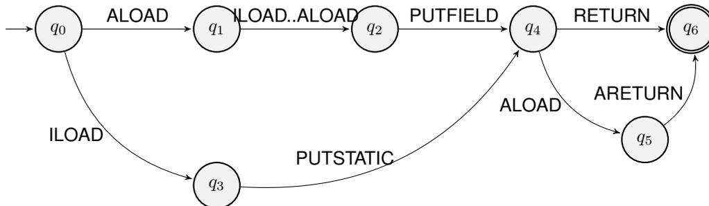
Figure 2.3: Finite automaton to detect simple setter methods
