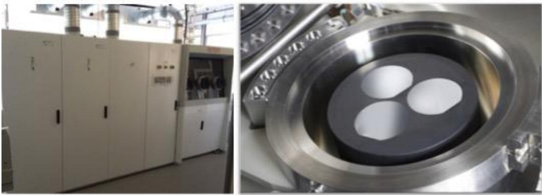
Figure 2-4 Aixtron 3x2 inch, close coupled showerhead (CCS) MOVPE system.
