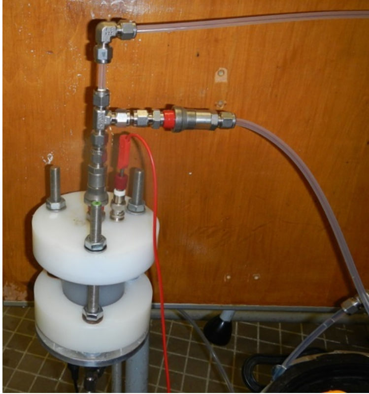
Figure 3.5: Cell of the permeameter / porosimeter apparatus equipped with electric connections for measuring the bulk conductivity of the medium and with tube derivations to monitor differential pressure at sample extremities.
