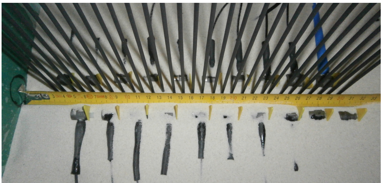
Figure 3.3: Picture of accelerometers and electrodes position within the measuring plane. The black circle marks the location of the source punch; the central line of the sandbox is materialised by the tip of the electrode array. It is framed by two parallel accelerometer lines shifted laterally by 1 cm.
