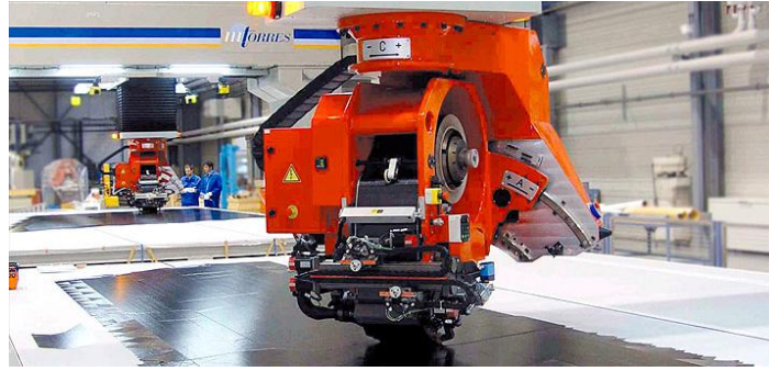
Figure 7 Typical automated tape laying system © MTORRES ( www.mtorres.com/ )
