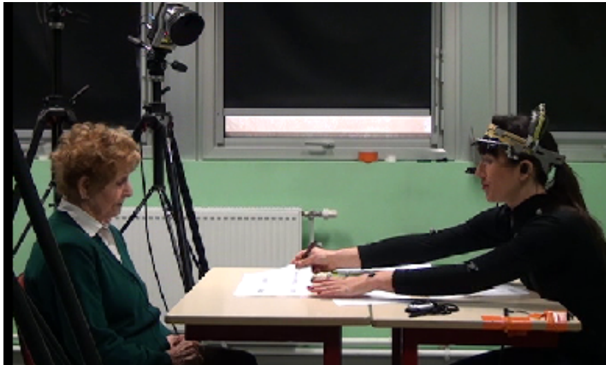
Figure 2.7 – Capturing the multimodal behavior of the human tutor during HHI. Movements of the upper limbs (head, arms and hands) are monitored by tracking 22 markers glued on these segments with a Qualysis ® mocap system. Gaze was tracked using a Pertech ® head-mounted eye tracker.
