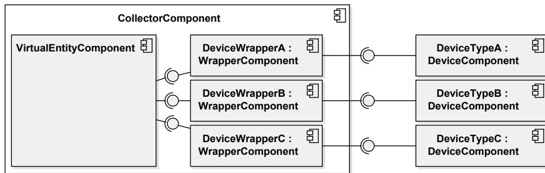
Figure 4.21: Collector Component Architecture Example
