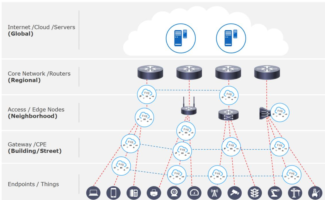
Figure 2.3: Fog Computing Conceptual Architecture (Source [63]).
