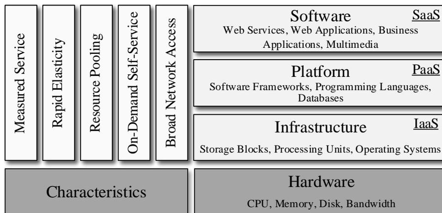
Figure 2.2: Traditional Cloud Computing Service Layers and Key Characteristics.
