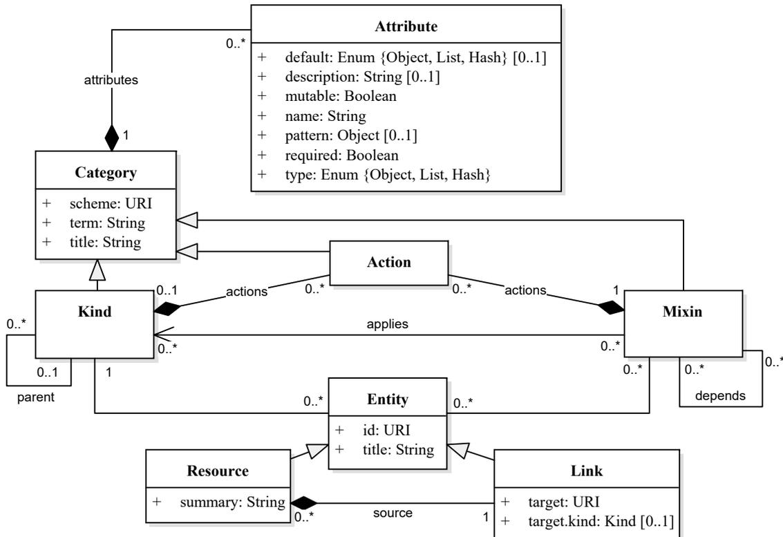
Figure 4.7: Open Cloud Computing Interface Core Model (Source [134])
