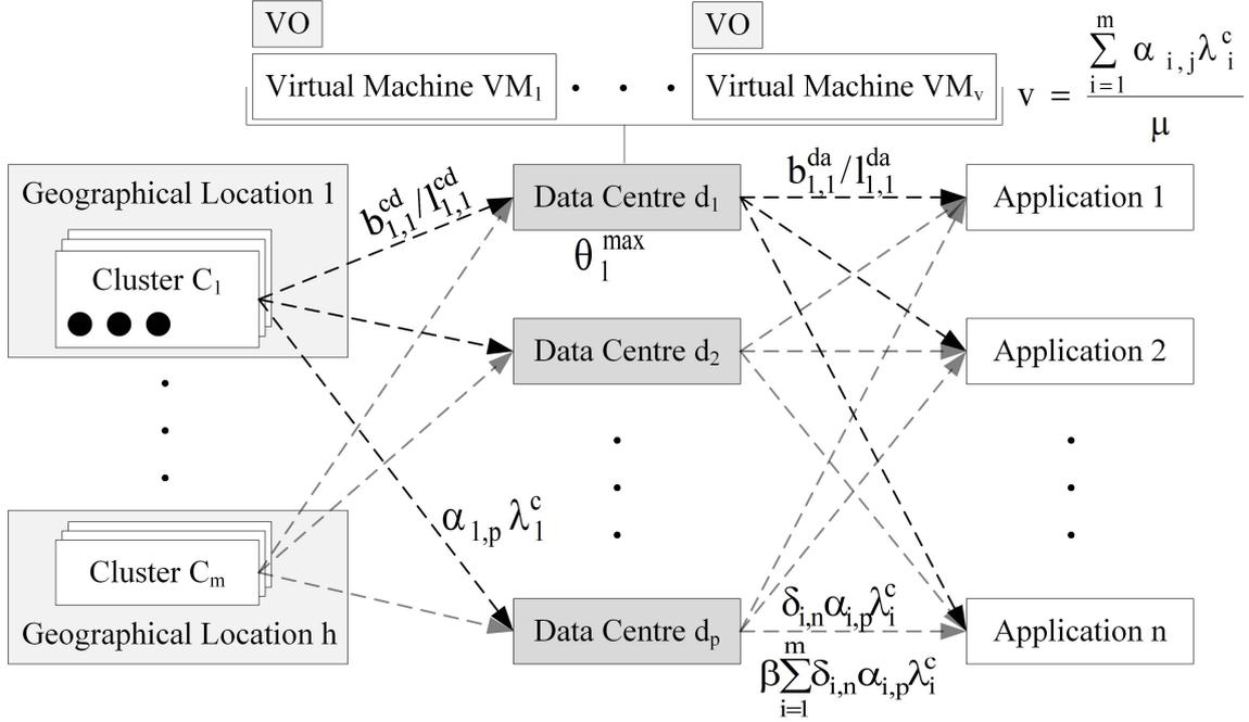
Figure 3.4: Network Model of the Placement Problem.
