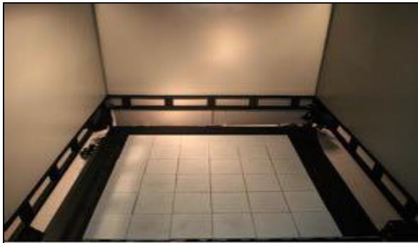
(a) The floor pressure-sensing interface.
