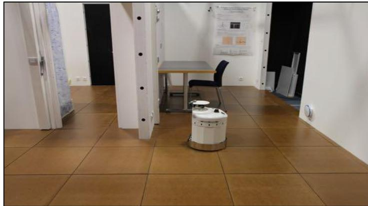
Figure 2.26 – PeKeeII robot communicating with an interactive sensing floor.
