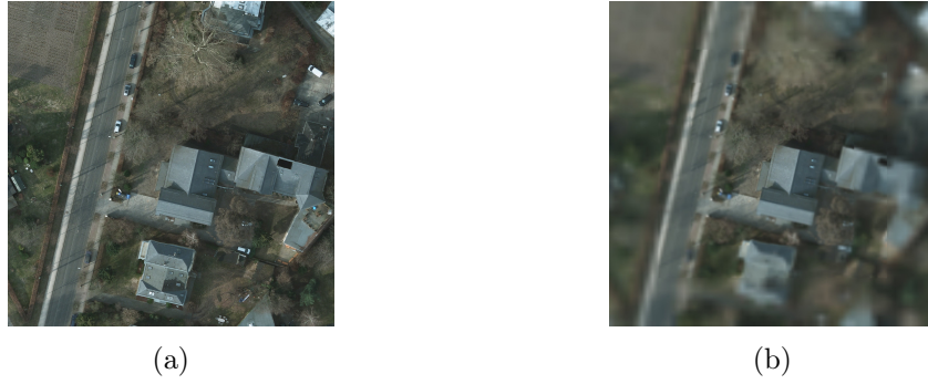
Figure 5.3: To classify the central gray pixel of this patch (and not to confuse it, e.g., with an asphalt road), we need to take into account a spatial context (a). However, we do not need a high resolution everywhere in the patch. It can be lower as we go away from the central pixel and still identify the class (b).
