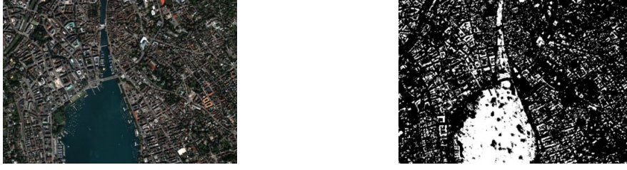
Figure 5.11: A CNN trained on a different dataset misclassifies most of Lake Zurich as a building.
