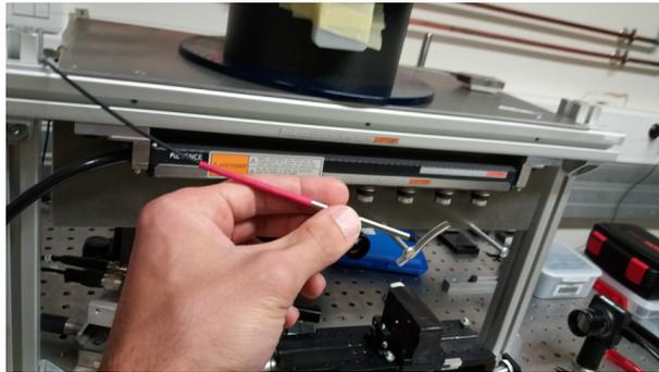
Figure 6.6: The flexible and miniature Kagomé DC probe.
