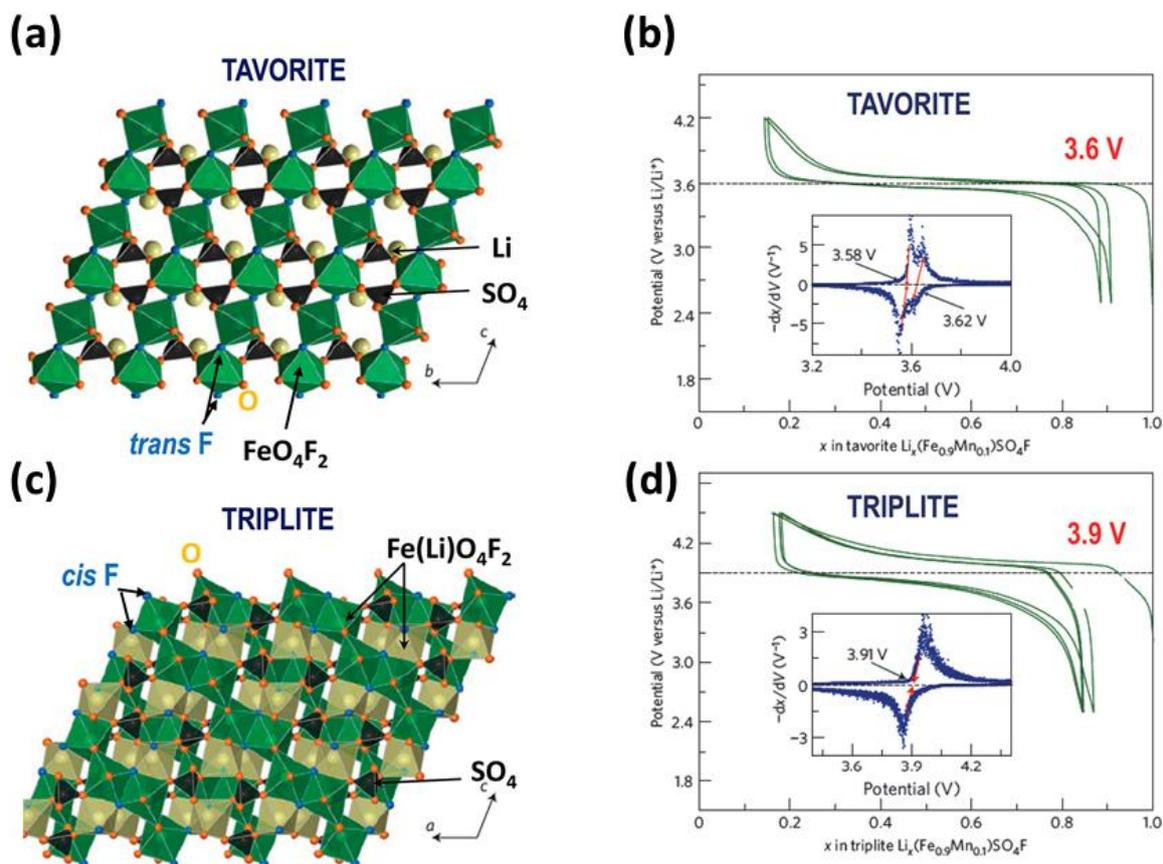
Figure 25 (a,c) Structure and (b,d) galvanostatic charge-discharge curves for tavorite- and triplite  $\text{LiFeSO}_4\text{F}$ .<sup>111</sup>
