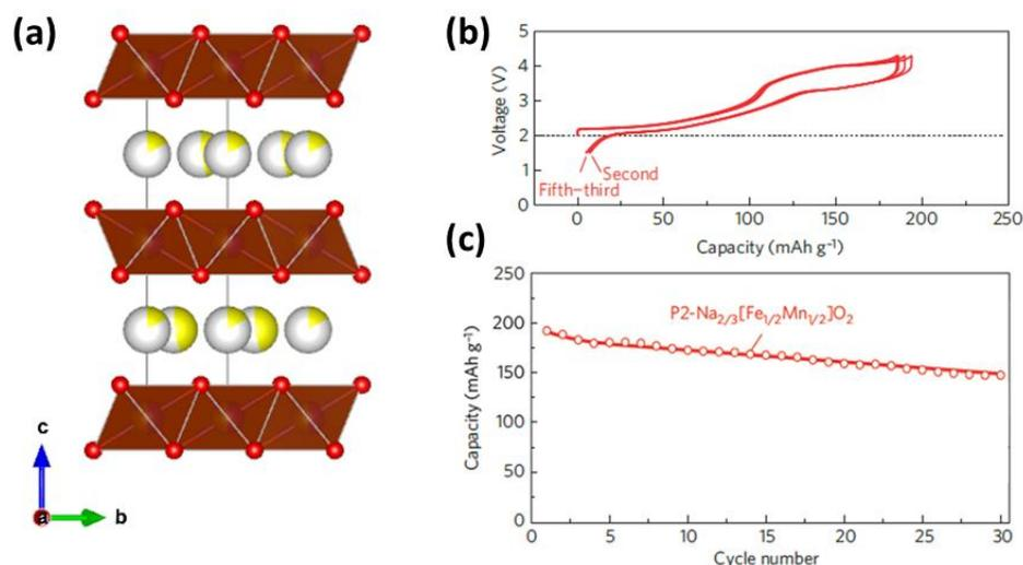
**Figure 11:** (a) Structure of the  $\text{P2-Na}_{2/3}[\text{Fe}_{1/2}\text{Mn}_{1/2}]\text{O}_2$  its (b) galvanostatic cycling and the corresponding capacity retention.<sup>45</sup>
