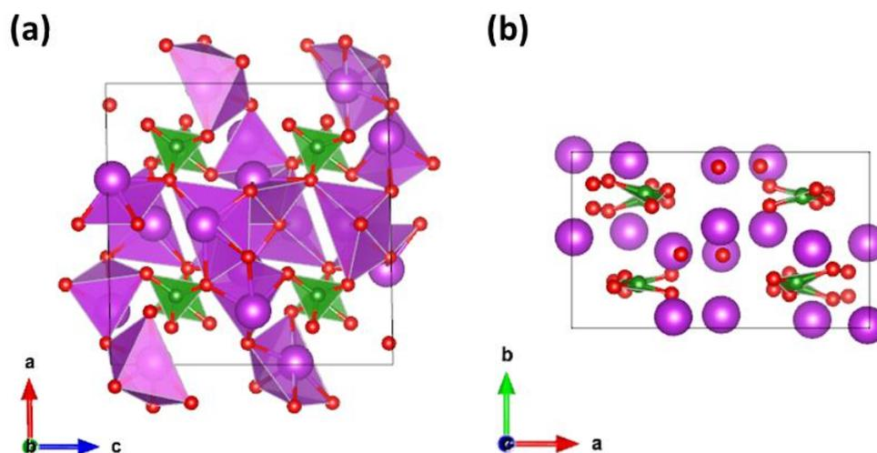
**Figure 75:** Crystal structure of  $\text{Bi}_4\text{B}_2\text{O}_9$  shown along the (a)  $b$ - and (b)  $c$ -axis. Bismuth atoms/polyhedral, boron and oxygen are shown in purple, green and red respectively.
