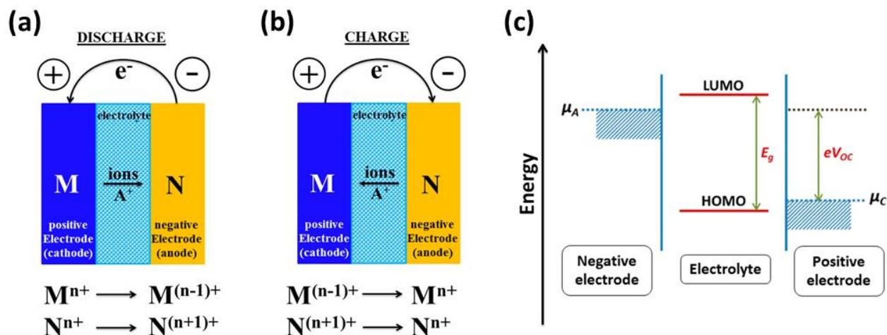
**Figure 5:** Schematic illustration of an electrochemical cell during (a) discharge and (b). (c) Energy diagram of an electrochemical cell. <sup>14,15</sup>
