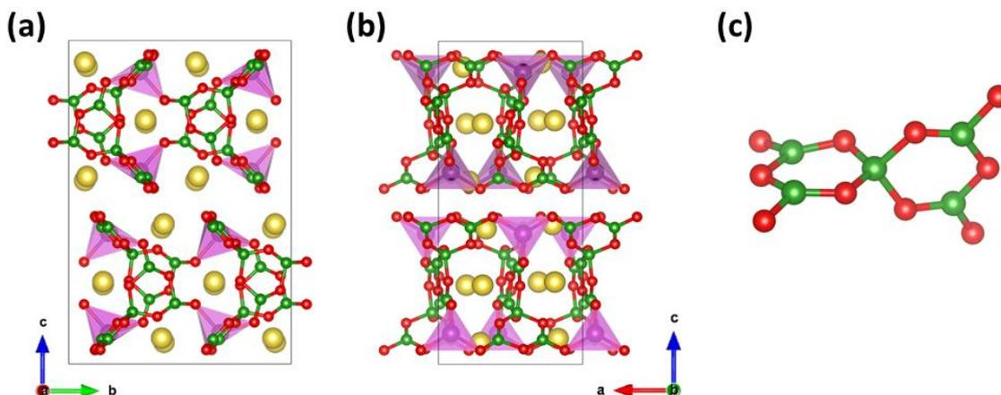
**Figure 64:** Structure of  $\text{Na}_3\text{FeB}_5\text{O}_{10}$  viewed along the  $a$ -axis (a) and the  $b$ -axis (b). Oxygen, boron, sodium and iron atoms indicated in red, green, yellow and pink respectively. (c) Pentaborate unit.
