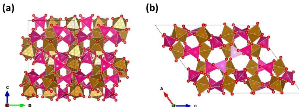
**Figure 14:** Crystal structure of the NASICON type compound  $\text{Fe}_2(\text{MoO}_4)_3$  along the (a)  $a$ - and (b)  $b$ -axis.  $\text{FeO}_6$  octahedra and  $\text{MoO}_4$  tetrahedra are shown in brown and purple respectively.
