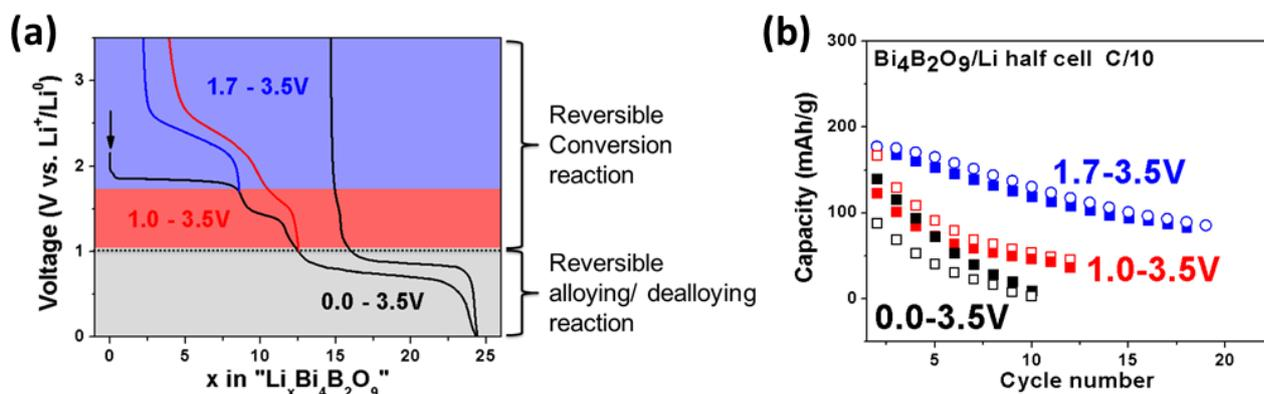
**Figure 95:** (a) Schematic illustration of the different voltage-composition curve of  $\text{Bi}_4\text{B}_2\text{O}_9$  versus Li depending on the lower cutoff potential referring to the conversion- and alloying part of the electrochemical reaction versus Li. (b) Capacity retention depending on the voltage window applied for galvanostatic cycling.
