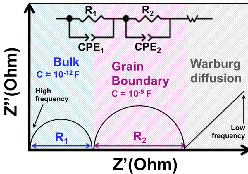
**Figure 98:** Representative Nyquist plot with the equivalent circuit to referring to bulk- and grain boundaries respectively. (Adapted from Ref.<sup>197</sup>).
