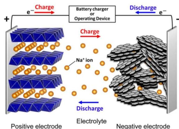
**Figure 8:** Schematic illustration of a Na-ion battery.<sup>31</sup>
