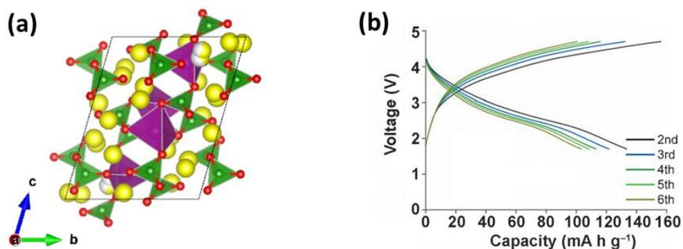
**Figure 34:** (a) Structure of  $\text{Li}_7\text{Mn}(\text{BO}_3)_3$  viewed along the *a*-axis. Oxygen, lithium boron and manganese are represented in red, yellow, green and purple respectively. (b) Galvanostatic charge-discharge curve for  $\text{Li}_7\text{Mn}(\text{BO}_3)_3$  between 4.7 and 1.7 V vs.  $\text{Li}^+/\text{Li}^0$  with 10 mA/g.<sup>153</sup>
