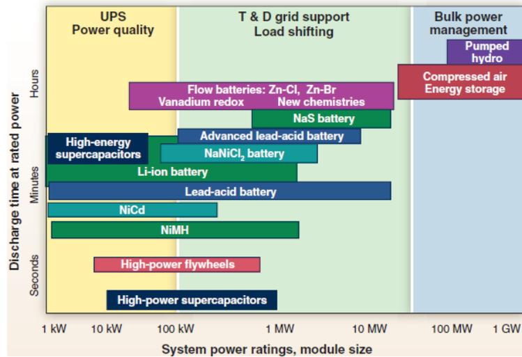
**Figure 3:** Comparison of discharge time and power rating for various electrochemical energy storage technologies.<sup>5</sup>
