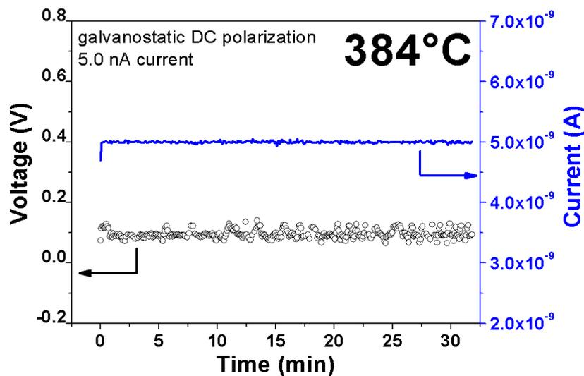
**Figure 93:** Representative galvanostatic DC polarization of  $\text{Bi}_4\text{B}_2\text{O}_9$ .
