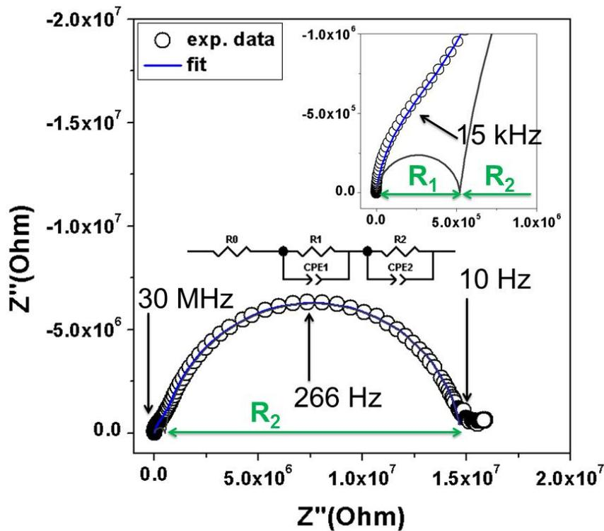
**Figure 92:** Representative AC complex impedance spectra of  $\text{Bi}_4\text{B}_2\text{O}_9$  measured at  $384^\circ\text{C}$  in air. The semi circles corresponding to the bulk- and grain boundary resistance are schematically drawn as grey lines, and the real resistance values are indicated with green arrows.
