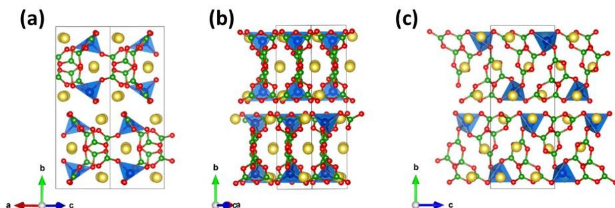
**Figure 66:** Structure of  $\text{Na}_3\text{CoB}_5\text{O}_{10}$  viewed along different crystallographic directions. Oxygen, boron, sodium and cobalt atoms indicated in red, green, yellow and blue respectively.
