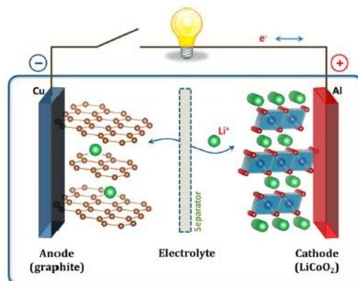
*Figure 7: Schematic view of a Li-ion cell based on a  $\text{LiCoO}_2$  cathode and a graphite anode.<sup>14</sup>*
