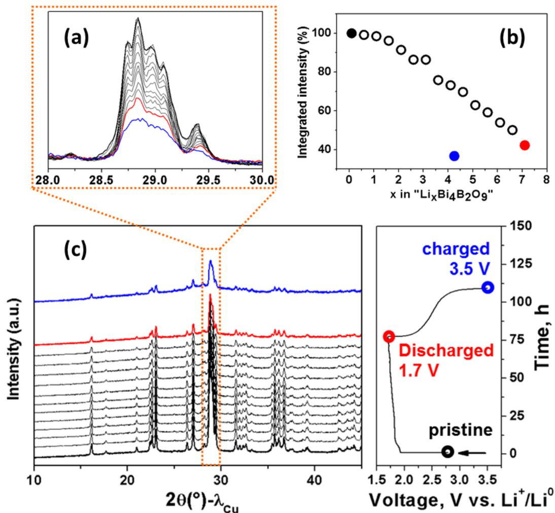
**Figure 89:** *In situ* XRD of the initial discharge/charge cycle of a  $\text{Bi}_4\text{B}_2\text{O}_9/\text{Li}$  half-cell cycled with a C/10 rate in a potential window between 1.7 and 3.5 V. XRD patterns were recorded every 0.1  $\text{Li}^+$ , however for reasons of clarity only every 5<sup>th</sup> pattern is shown in (c). A magnification of the main reflections is presented in (a) and their integrated intensity of the main reflection is shown in (b).
