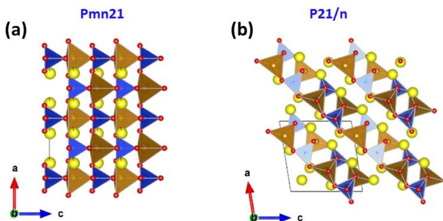
**Figure 22:** Two known polymorphs of  $\text{Li}_2\text{FeSiO}_4$  crystallizing in (a)  $P2mn21$  and (b)  $P21/n$  space group.  $\text{FeO}_4$  tetrahedra,  $\text{SiO}_4$  tetrahedra and  $\text{Li}$  are drawn in brown, blue and yellow respectively.
