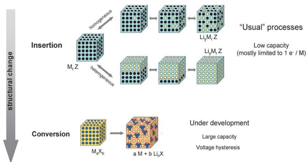
**Figure 26:** Schematic illustration of insertion and conversion type reaction investigated as electrode materials for Li- and Na-ion batteries.<sup>15</sup>
