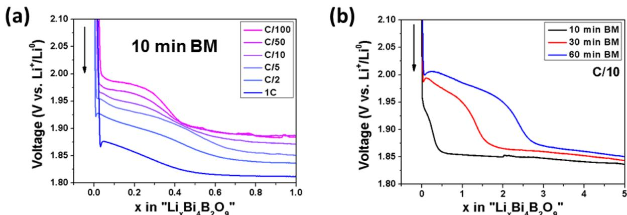
**Figure 90:** Initial discharge of  $\text{Bi}_4\text{B}_2\text{O}_9$ /carbon composite. In (a) the influence of different C-rates is shown for a milling time of 10 min, whereas in (b) the impact of the milling time is presented.
