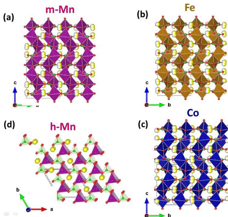
**Figure 31:** Crystal structures of  $\text{LiMBO}_3$  for (a)  $M = \text{Mn}$  (monoclinic), (b)  $\text{Fe}$ , (c)  $\text{Co}$  and (d)  $\text{Mn}$  (hexagonal). Oxygen, lithium and boron atoms are shown in red, yellow and green respectively.
