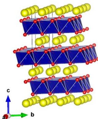
**Figure 10:** Schematic view of the crystal structures of layered  $\text{LiCoO}_2$  with Li-, Co- and O atoms drawn in yellow, blue and red respectively.
