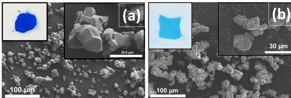
**Figure 38:** Representative SEM images of (a)  $\alpha\text{-Li}_6\text{CuB}_4\text{O}_{10}$  and (b)  $\beta\text{-Li}_6\text{CuB}_4\text{O}_{10}$ . Insets show a magnified view on the crystallites and a colored picture of the as-prepared powder.
