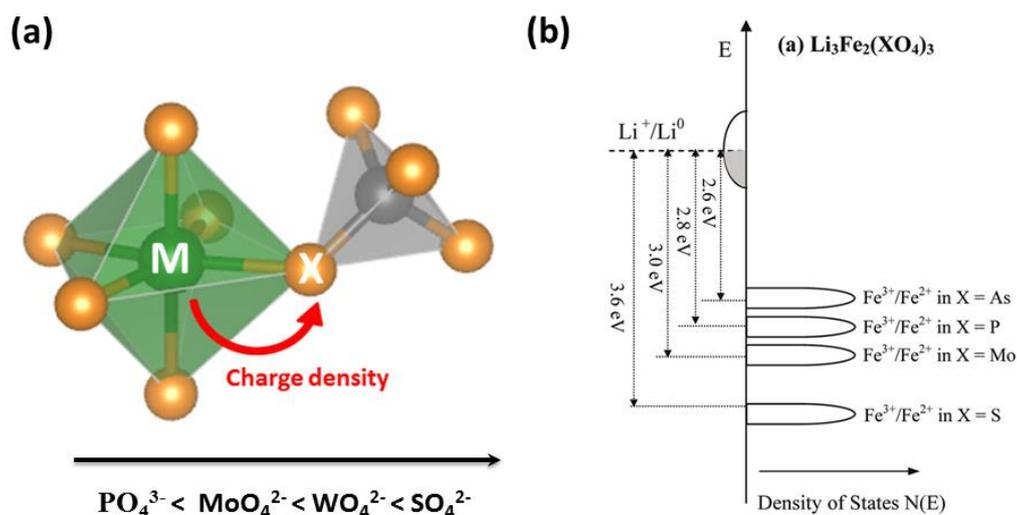
**Figure 15:** Schematic representation of the inductive effect. (a)  $\text{MO}_6$  octahedra connected over one bridging oxygen to the  $\text{XO}_4$  tetrahedra. (b) Depending on the electronegativity of the polyanionic group, the redox potential of the  $\text{Fe}^{3+}/\text{Fe}^{2+}$  can be shifted up from 2.8 to 3.6 V vs.  $\text{Li}^+/\text{Li}^0$ .<sup>71</sup>
