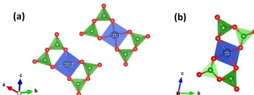
**Figure 41:** View of the  $[\text{Cu}(\text{B}_2\text{O}_5)_2]^{6-}$  structural unit in (a)  $\alpha\text{-Li}_6\text{CuB}_4\text{O}_{10}$  (Cu1 and Cu2) and (b)  $\beta\text{-Li}_6\text{CuB}_4\text{O}_{10}$  (Cu1). Copper, boron and oxygen atoms are shown in blue, green and red respectively.
