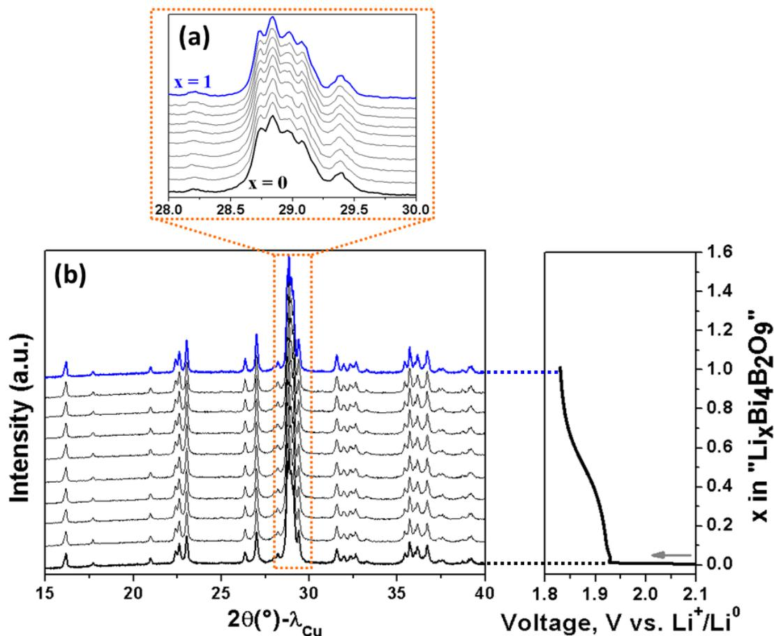
**Figure 88:** In situ XRD of the initial discharge of a  $\text{Bi}_4\text{B}_2\text{O}_9/\text{Li}$  half-cell cycled with a C/10 rate till a Li uptake of  $x = 1.0$ . XRD patterns were recorded every  $0.1 \text{ Li}^+$ . A magnification of the main reflections is presented in (a) and an overview over the whole XRD pattern and the corresponding voltage-composition curve is shown in (b).
