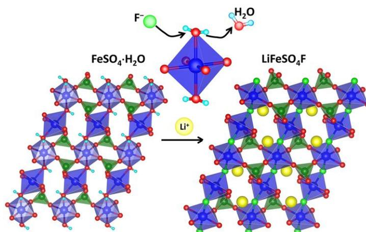
**Figure 24:** Structural relationship between the precursor  $\text{FeSO}_4\cdot\text{H}_2\text{O}$  and the *tavorite*  $\text{LiFeSO}_4\text{F}$ .<sup>107</sup>
