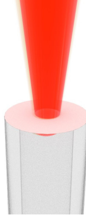
Figure 3.6 – Principle of laser ablation : a \text{CO}_2 laser is highly absorbed in the first tens of microns of silica.
