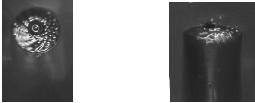
Figure 3.17 – A “pencil” shape fibers observed with a microscope. the rough surface far from the mirror reflects the shooting pattern .The diameter of the fiber is 125\text{ }\mu\text{m} , the concave depression RoC is 10\text{ }\mu\text{m} . SEM image of such a fiber is displayed on the front page of this chapter.
