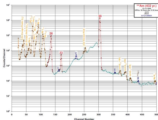
**Figure 5.7 :** Gamma-ray spectrum of  ${}^{241}\text{Am}$  taken from the website [www.radiochemistry.org](http://www.radiochemistry.org)
