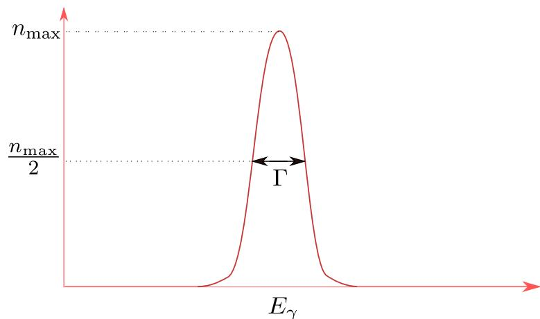
**Figure 2.10 :** Illustration of the detector's resolution around a peak of energy  $E_\gamma$
