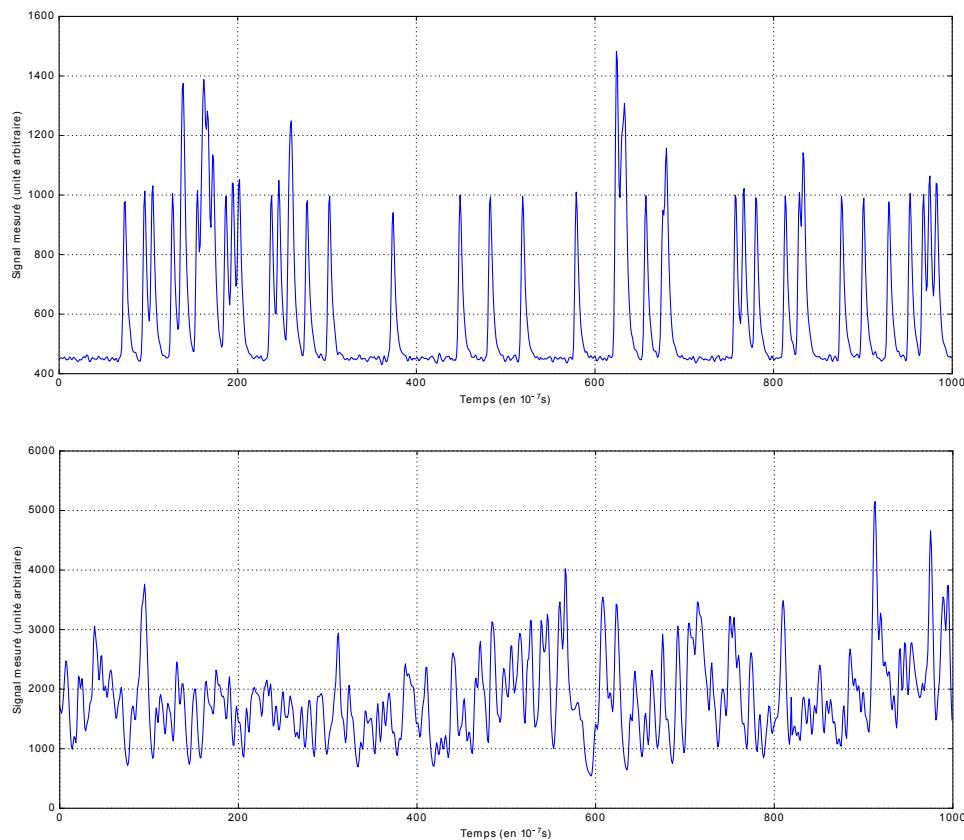
**Figure 2.13 :** Two shot-noise processes from  $\gamma$ -spectroscopy measurements: the radioactive source is a mixture of Americium 241 and Plutonium 238. The intensity rates are respectively of  $5.10^5$  et  $4.10^6$  counts by second in the upper and lower figures
