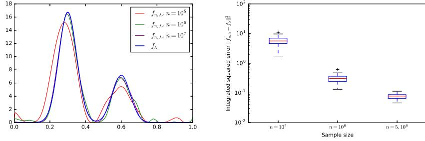
**Figure 5.5** : Left: Estimation of  $f_\lambda$  for  $n \in \{10^5, 10^6, 10^7\}$  using Algorithm 2. Right: Boxplot of the Integrated Squared Error  $\|\hat{f}_{n,\lambda} - f_\lambda\|_2^2$  for  $n \in \{10^5, 10^6, 5.10^6\}$  and 100 independent runs of Algorithm 2 over independent input data sets
