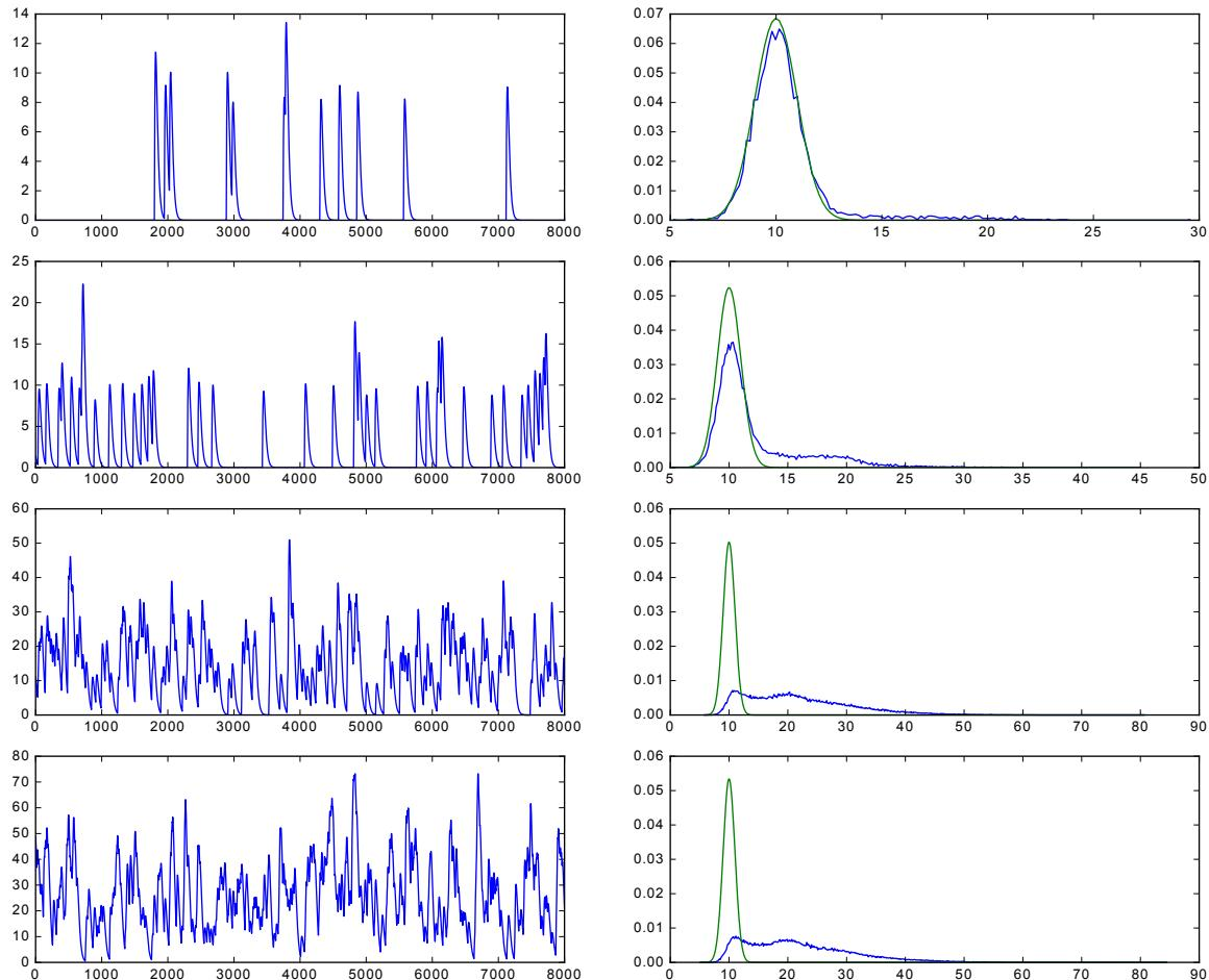
**Figure 2.14 :** Left: Sample paths of simulated shot-noise processes with triplet  $(\lambda, f, h)$  for  $\lambda \in \{0.2, 1, 5, 10\}$  for a same impulse response  $h$  and the same marks' density  $f$ . Right: Histogram of the local maxima associated to a sample of the shot-noise process of size  $n = 5.10^6$
