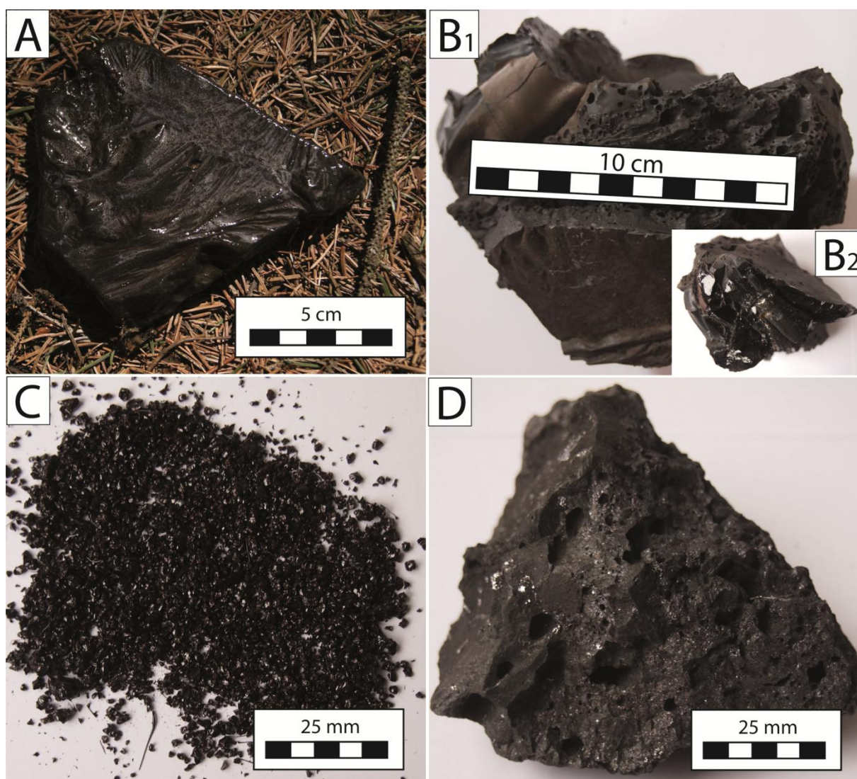
FIGURE 4.1 Macroscopic pictures presenting slags selected for this study.
