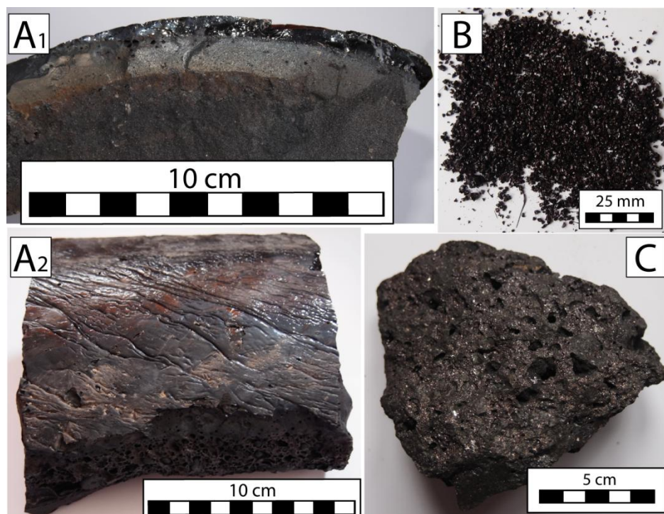
FIGURE 3.7 Modern slags (A1 and A2: shaft furnace slag, B: granulated slag, C: lead slag).
