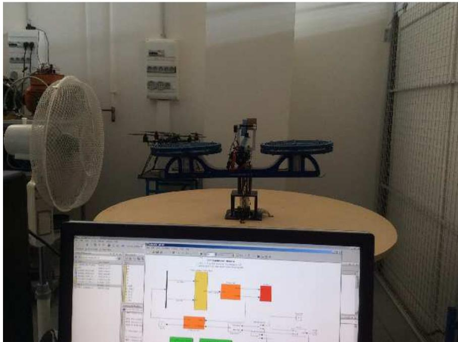
Figure 10.1 – **Top.** Scheme of Quanser 3DOF tandem helicopter; **Bottom.** Photo of the experimental set-up (with the fan on the left hand side, producing perturbations as wind gusts, and the control PC on foreground, with Matlab/Simulink software).
