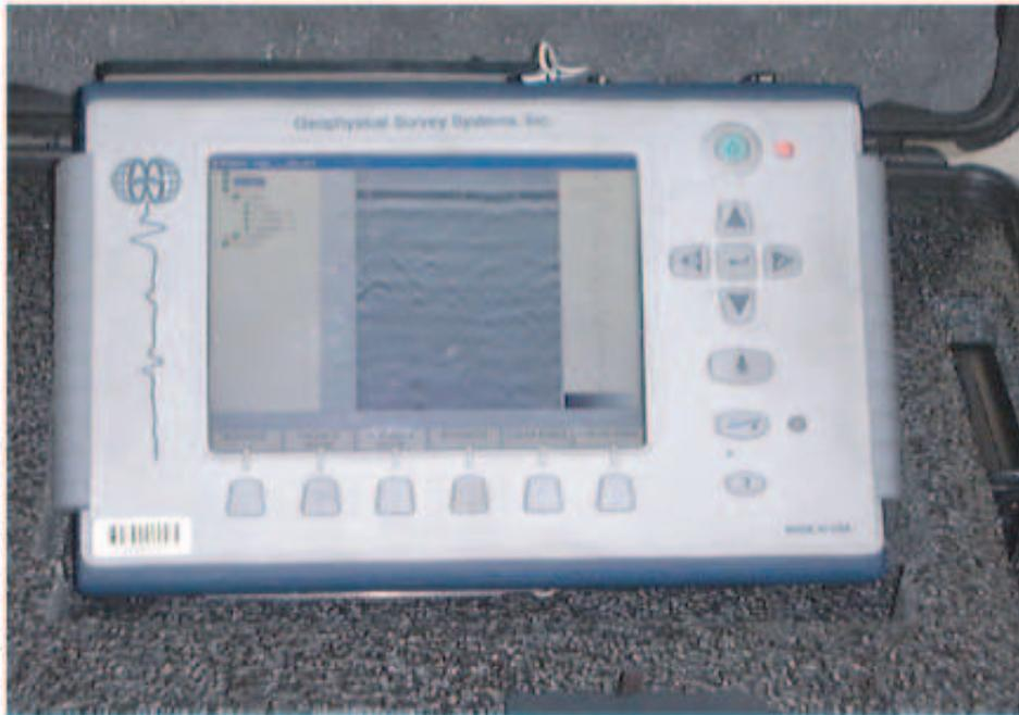
Figure 1.1: Example of an impulse GPR (SIR-3000) [5]
