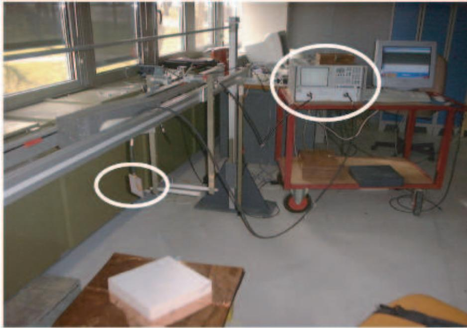
Figure 1.2: Example of a step frequency GPR [5]
