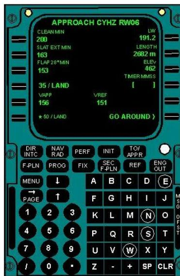
Figure 3.3: Multifunction Control Display Unit (MCDU) [Wikipedia, 2015d]
