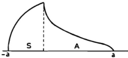
Figure 1.14 Local traction distribution according to Carter Theory (2D model: S is an area of slip; A is an area of adhesion.)
