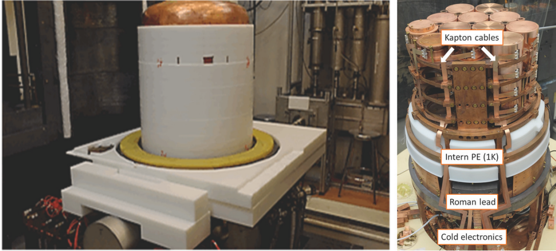
Figure 2.12. – Picture of the external (left) and internal (right) PE shields added in EDELWEISS-III.
