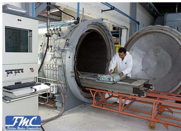
Figure 19 : A pre-preg part under vacuum going into the FMC autoclave, [91].
