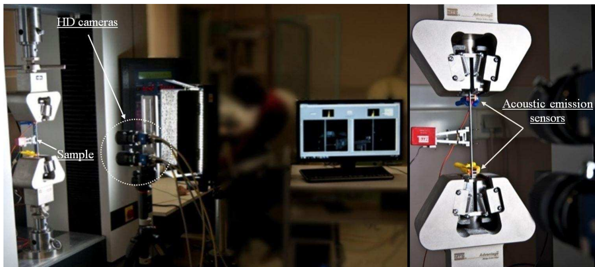
Figure 37 : Test set-up to measure intralaminar tensile cracking.
