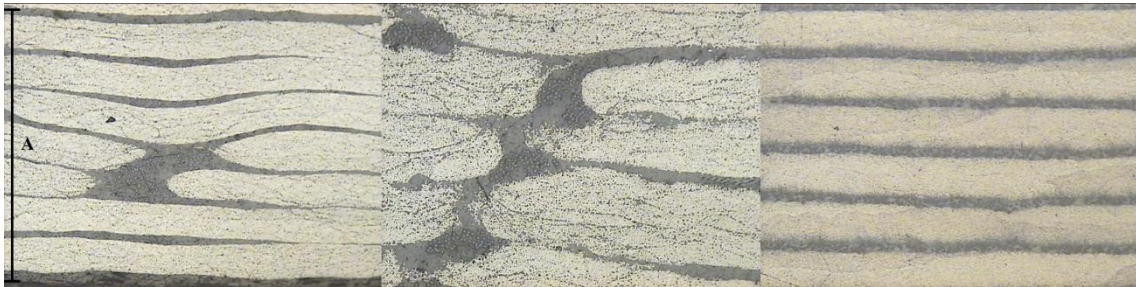
Figure 55: Optical microscope observation of UD samples, left to right, Infused, RTM and Pre-preg materials (dimension A is approximately 1.5 mm, for all three materials).
