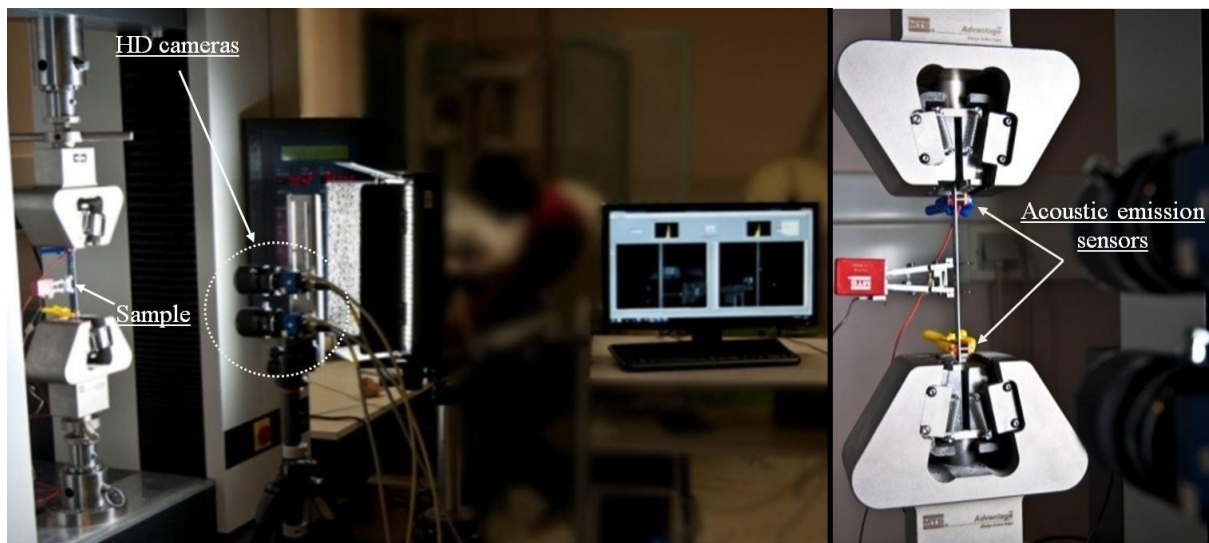
Figure 37 : Test set-up to measure intralaminar tensile cracking.
