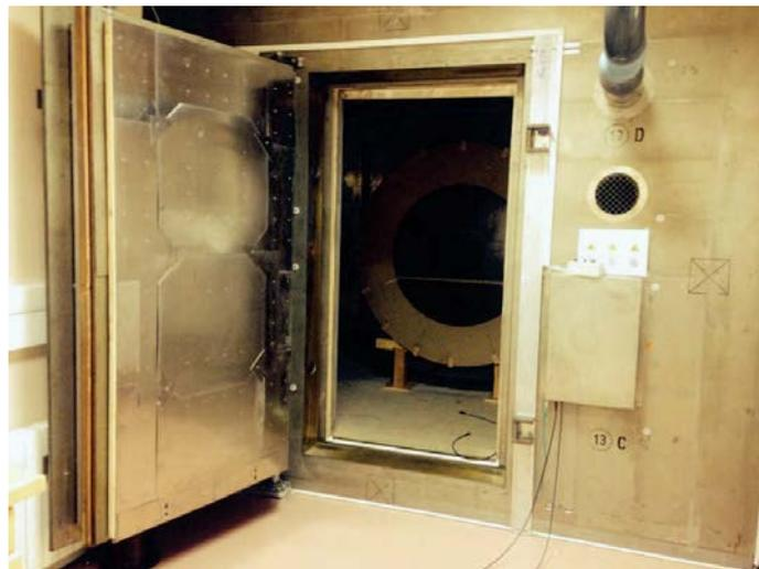
Figure 3.19: Magnetically shielded room at SPEC/CEA Saclay.
