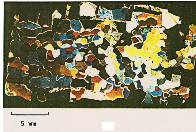
Figure 4.2: Grain boundaries in atmospheric ice accumulated at -4.8^{\circ}\text{C} [106]
