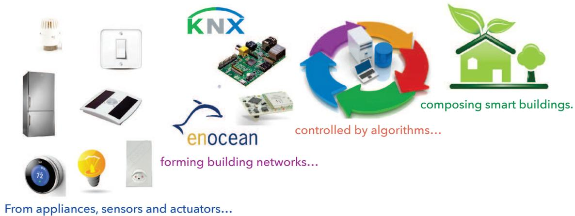
**Figure 1.1:** A couple of stages are required until energy savings and comfort improvement can be obtained in Smart Buildings. Control algorithms rely on functionalities offered by building networks themselves composed of smart things. They range from home appliances to sensors and actuators.
