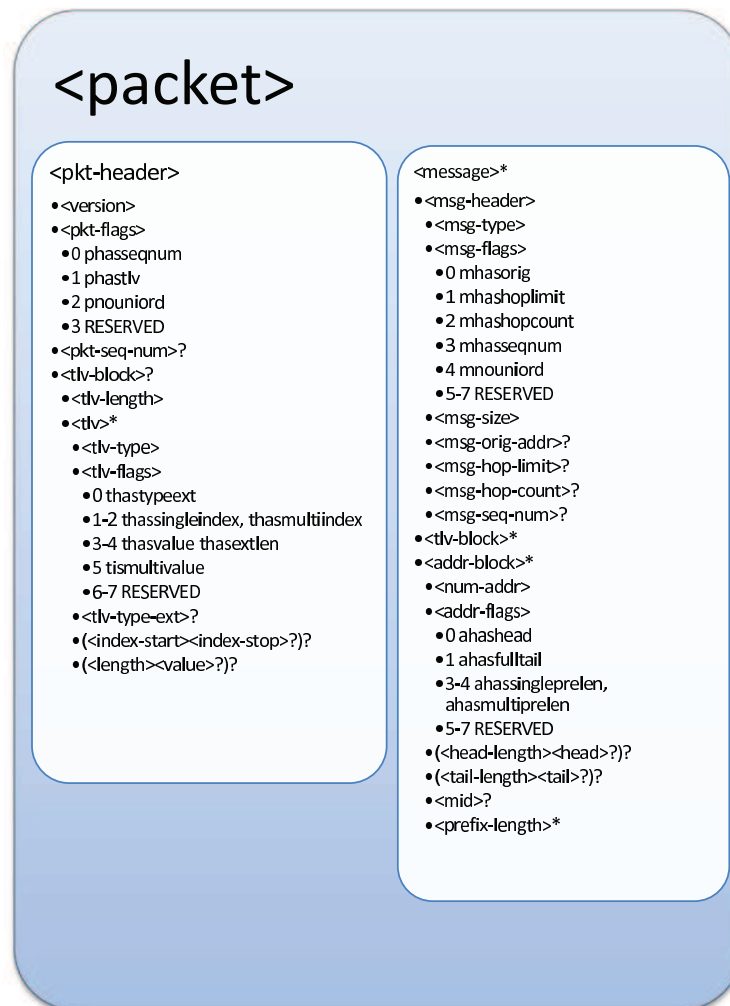
Figure 5.1: Generalized MANET Packet Format
