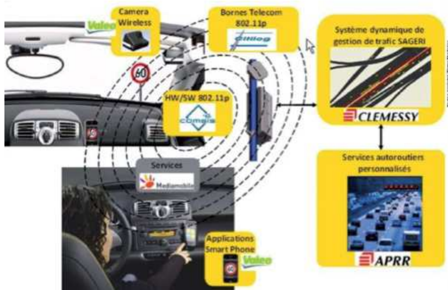
Figure 5.1: Cooperative driving based on integrated information technologies [155].
