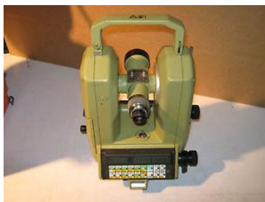
Figure 4.15 - Theodolite used for laser calibration
