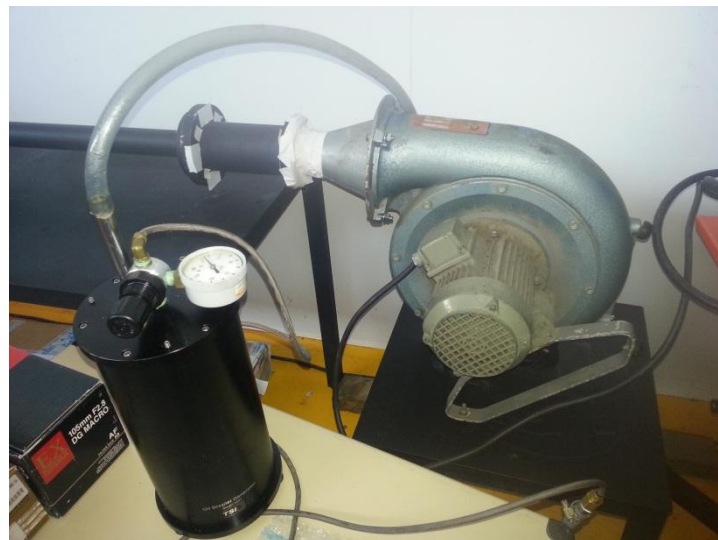
Figure 4.44 - PIV feeding system
