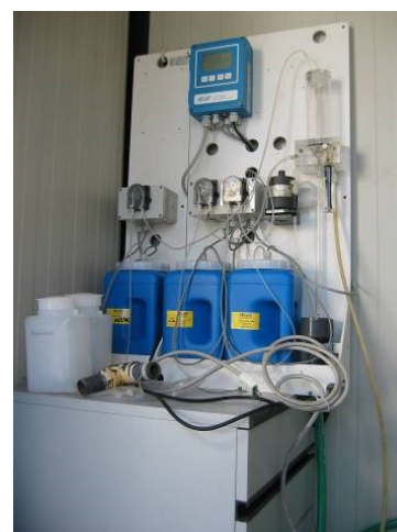
Figure 3-8: BIOX and chlorination treatments: (a) BIOX signal trend and residual oxidant concentration in seawater measured with the on-line instrumentation based on DPD colorimetric method, (b) AMI Codes (SWAN) colorimetric device.
