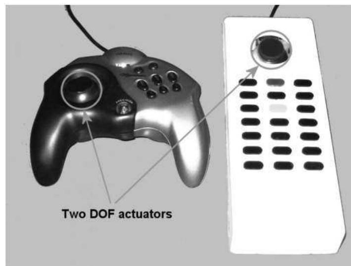
Figure 2.9: Handheld haptic device. A remote control including a 2DoF force-feedback joystick [OO04].
