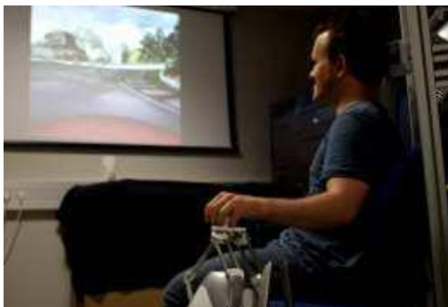
Figure 3.4: The user, comfortably installed on our device, is experiencing passive navigation enhanced by a haptic effect of motion.
