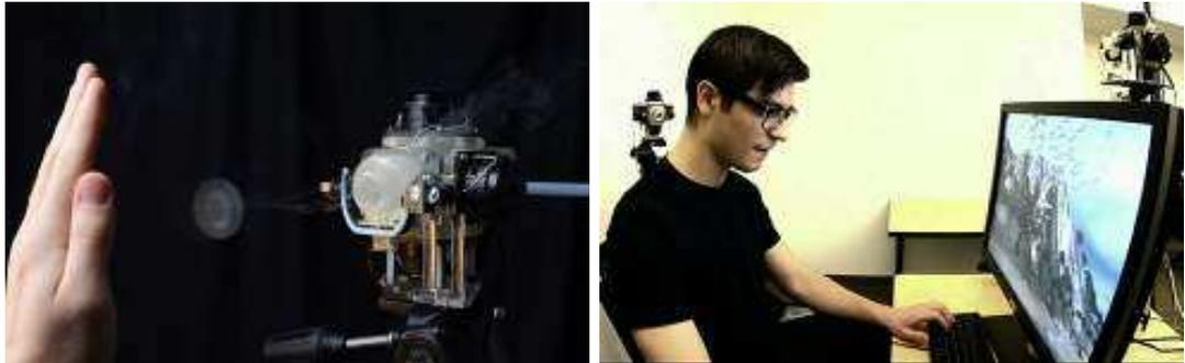
Figure 2.11: Desktop haptic device. The AIREAL, a contact free tactile interface [SPGI13].
