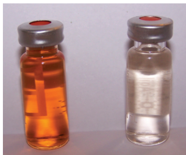
Figure 4.20: Effect of acetic acid on iron under biogas ( right ) and air ( left )
