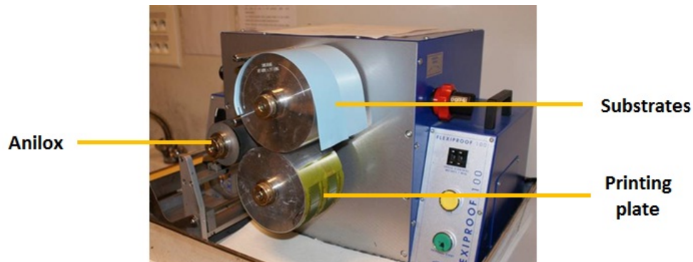
Figure 7.7: Flexiproof 100 laboratory printing tester
