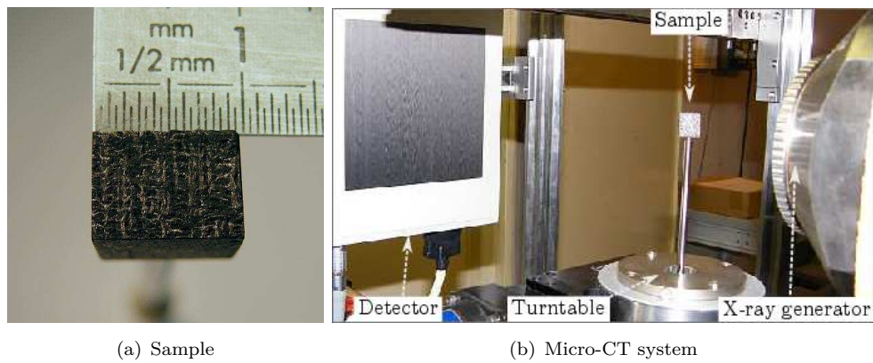
FIGURE 8.7: Micro-CT: A cubic sample of a material composed of carbon fibers in a matrix of carbon and the acquisition system. Courtesy of M.Costin.
