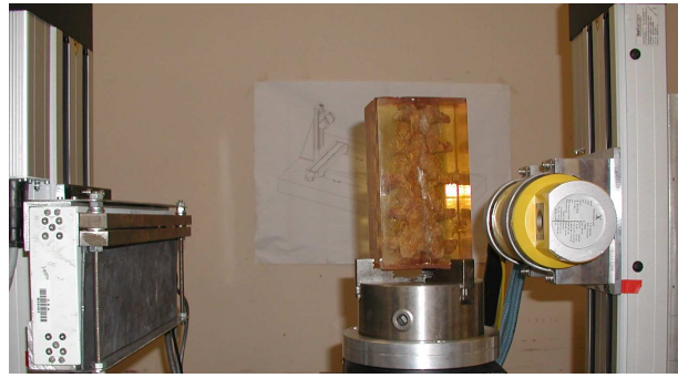
FIGURE 8.2: Acquisition system for the spine object. From right to left: X-ray tube, gantry and sample, linear detector.
