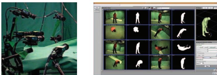
Figure 2.3: A commercial markerless capture system by 4DViews, based on work by [AMR<sup>+</sup>07]. The subject is isolated from the background (*right*) in camera view. A 3D reconstruction is computed on the fly, with textures projected from camera views.
