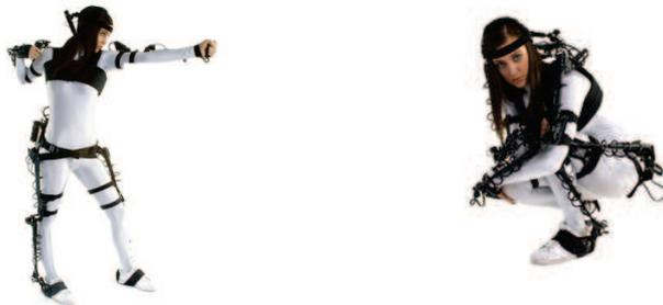
Figure 2.1: Gypsy 5, by Animazoo, an example of a *mechanical* motion capture device.
