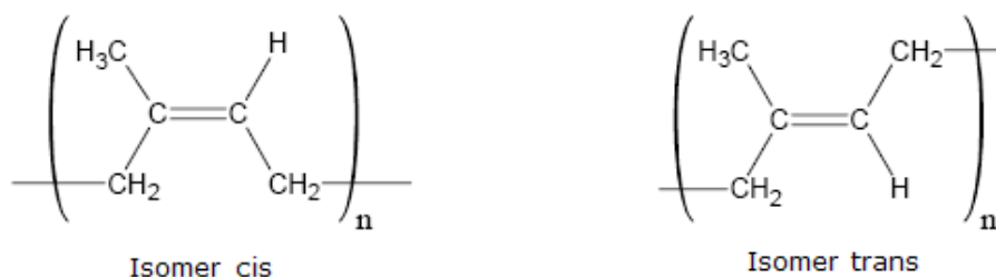
(b) cis- and trans- isomers of polyisoprene
