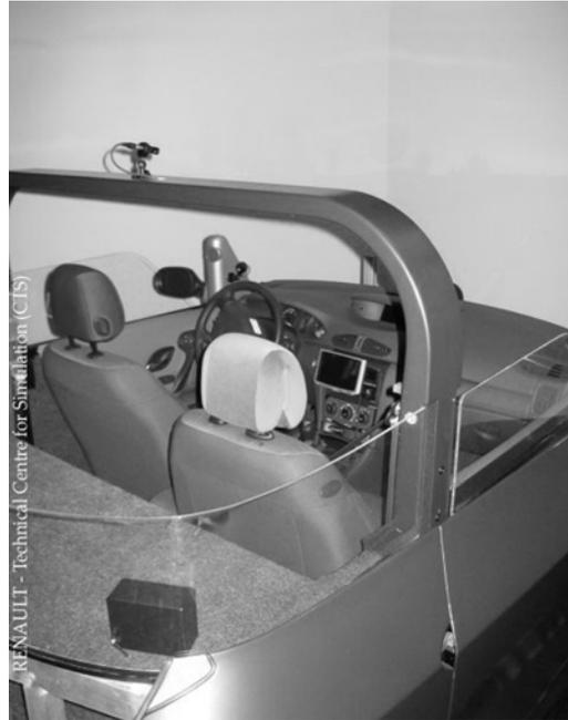
**Fig 2:** Picture of the CARDS simulator, with mid-console assistance display.
