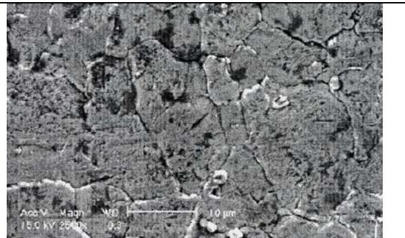
**Figure IV-20: Oxide scale granular morphology: Micrograph of specimen oxidized in air at 900°C and deformed at 800°C [Mou1].**
