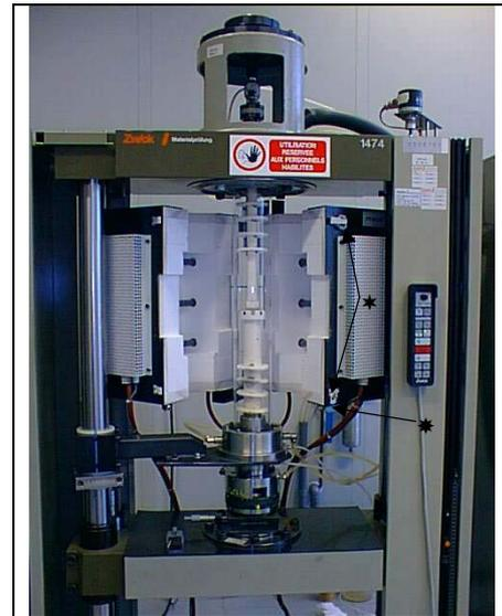
**Figure IV-23: Opened Pyrox Furnace.**
