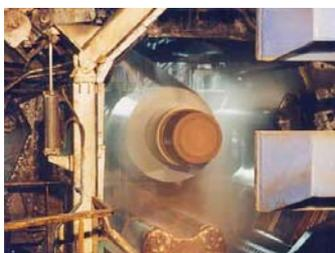
**Coiling:** Finally steel sheets, 2 to 5mm thick and up to 700m long, are coiled for storage.
