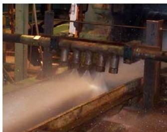
**RSB descaling (Roughing Scale Breaker):** At the exit of the furnaces, the primary scale must be removed, not to be irreversibly embedded in the metal and form important defects. To avoid this, a descaling ramp is installed. Nozzles project water under-pressure (150 bars) on the product. A combination of thermal and mechanical effects removes the thick primary scale before the first roughing mill stand.
