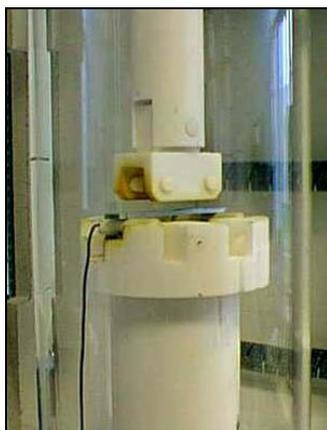
**Figure IV-24: Specimen installation in the silica tube.**
