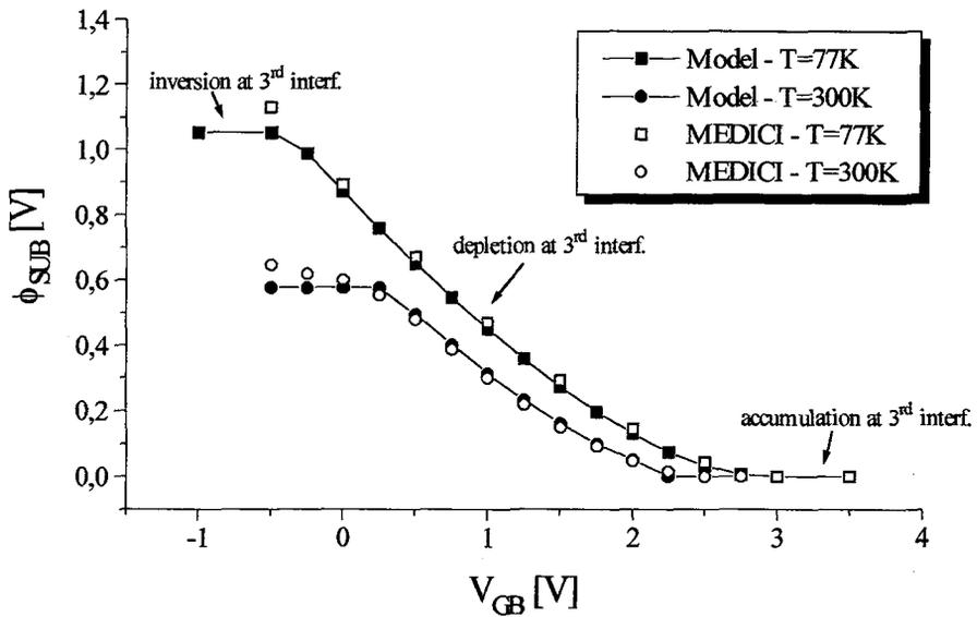
figure 2 - Comparison between analytical model and MEDICI simulation at room temperature and at 77 K.
