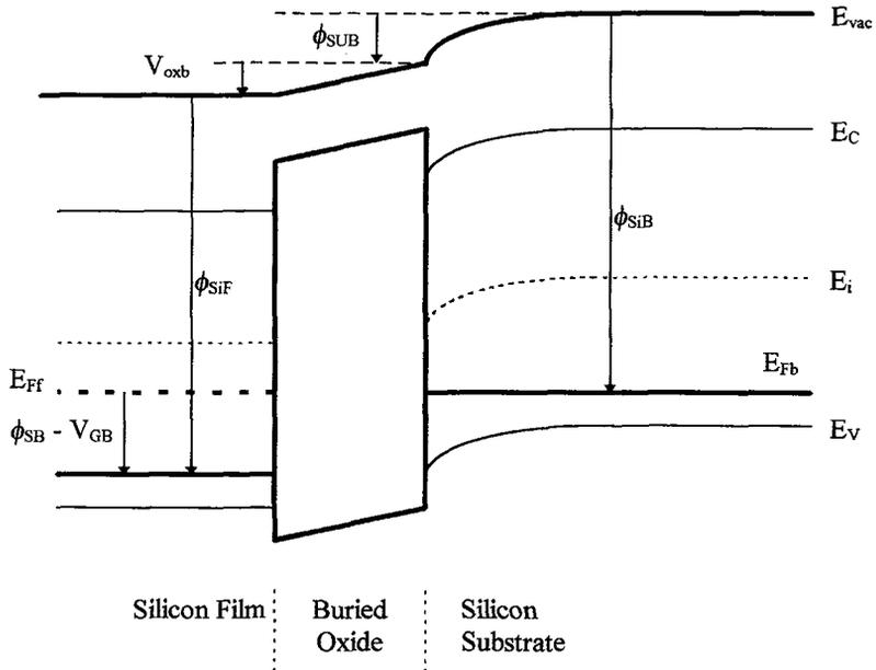
figure 1 - Band Diagram for pseudo-MOS structure
