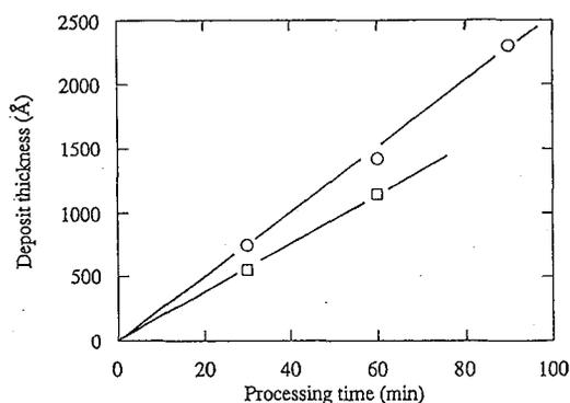
Figure 4 : Dependence of the copper film thickness on the processing time. The experimental conditions were : total pressure  $10^{-1}$  Torr, gas flow 1 sccm, ratio  $O_2/Cu(acac)_2 = 1.5$  and substrate temperature 350°C. (○) under UV illumination, (□) without photoassistance.
