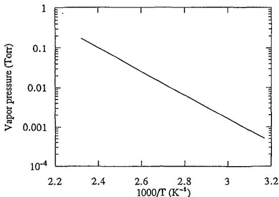
Figure 1: Dependence of the copper acetylacetonate  $\text{Cu}(\text{acac})_2$  vapor pressure on the temperature.
