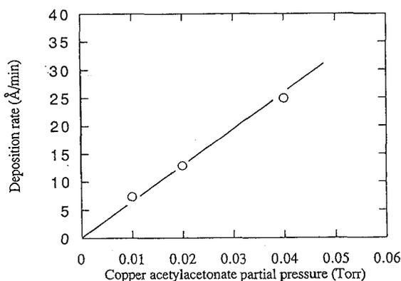
Figure 5 : Dependence of the deposition rate on the  $Cu(acac)_2$  partial pressure. The substrate temperature was 350°C, the gas flow 1 sccm and the ratio  $O_2/Cu(acac)_2$  was 1.5.
