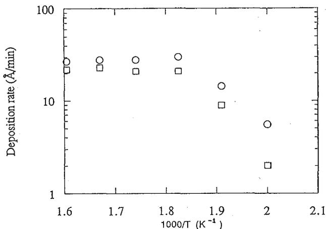
Figure 6 : Dependence of the deposition rate on the substrate temperature. The total pressure was  $10^{-1}$  Torr, the gas flow 1 sccm and the ratio  $O_2/Cu(acac)_2$  was 1.5. (○) under UV illumination, (□) without photoassistance.
