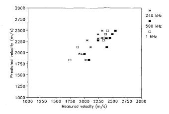
Figure 1. Velocity of the fast compressional wave compared to predictions of the Biot theory.
