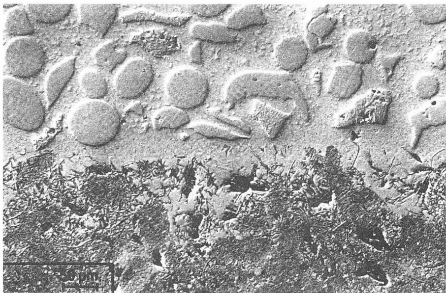
Fig. 1 : MMC produced on a cast iron; reinforcing particles : tungsten carbides.
