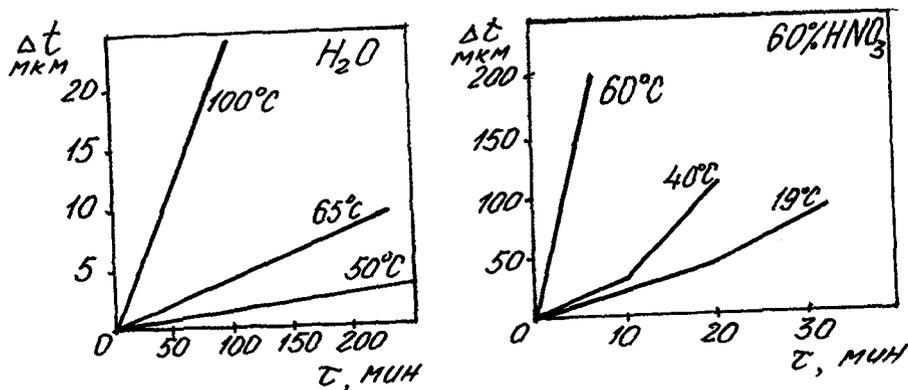
Fig. 6. Kinetic curve of LBO dissolution in hot water and in concentrated  $HNO_3$
