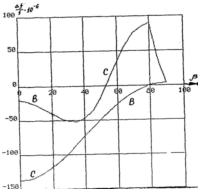
Fig. 7. Dependence of temperature-frequency coefficient of frequency of B and C nodes on LBO crystal on the angle of cut  $YX1/\beta$  of a piezoelectric element
