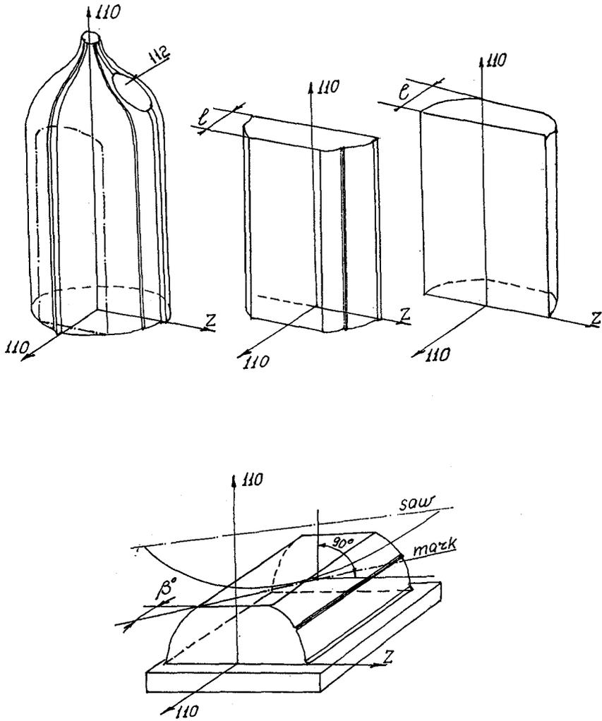
Fig. 5. Technology of cutting LBO crystal boule  $[110]$  into  $yx1/\beta$
