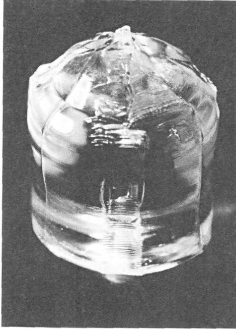
Fig. 2. "As grown" crystal LBO in the direction  $YX1/53^\circ$
