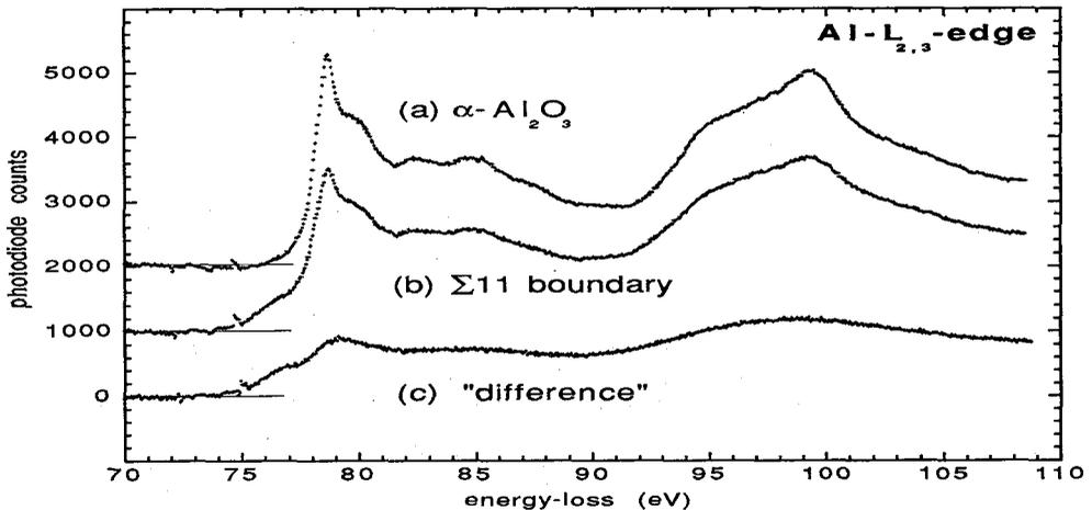
Figure 6: Al  $L_{2,3}$ -edge ELNES of the  $\Sigma 11$  grain boundary in a sapphire bicrystal. The spatial-difference ELNES reveals information about the bonding and coordination of the aluminium atoms at the boundary.
