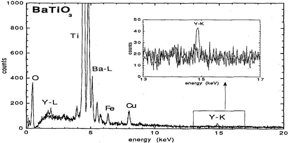
Figure 3: EDX spectra from a grain boundary and bulk BaTiO<sub>3</sub> revealing Y segregation.
