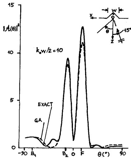
Fig.2 Bistatic cross section
